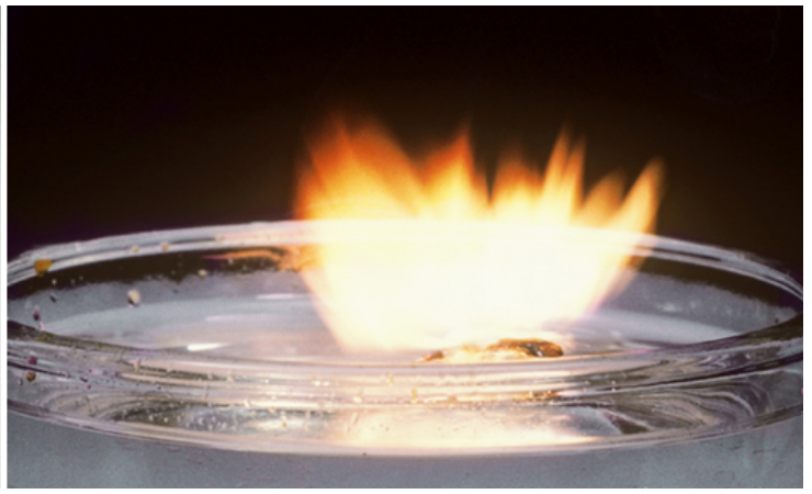
Left: The chemical element sodium is a silvery metal that is soft enough to cut with a knife. Right: When sodium is added to water a vigorous chemical reaction produces explosions of gas that often burst into flames.
