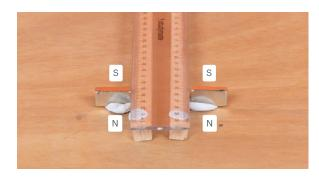
Note that when placing the magnets on the outside of the accelerator, the orientation of the poles should be parallel to the accelerator. This means that the poles should face towards and away from the entry of the accelerator, rather than inwards.
