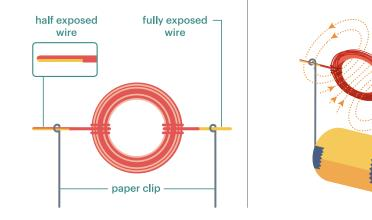
2. The electric current creates a magnetic field around the coil.
