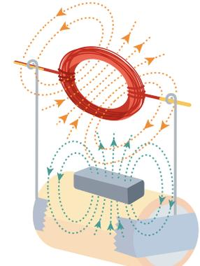
*In order for the coil to continue to spin, the circuit containing the copper coil must be broken. This prevents the magnetic field from the copper coil from permanently aligning with the magnetic field from the magnet. When the circuit is broken, momentum will allow the coil to complete its rotation, at which point the circuit reforms.*
